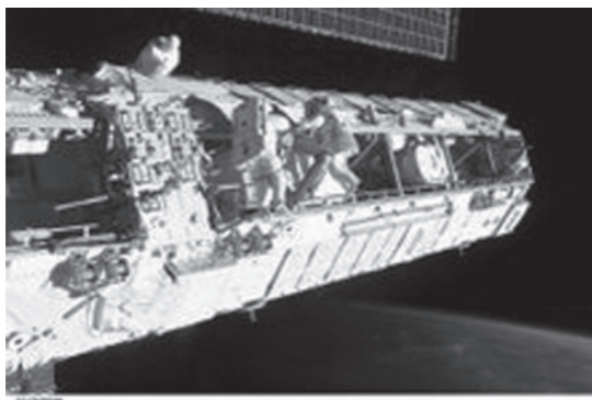
P1 Truss Being Installed During Space Shuttle Mission STS-113/ISS-11A
