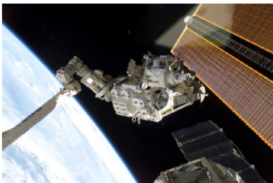
The MBS is moved by Canadarm2 for installation on the ISS during space shuttle mission STS-111/ISS-UF2.
