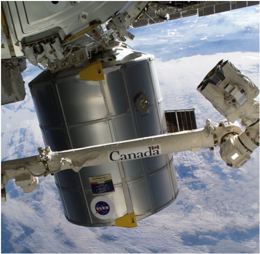
MPLM Raffaello is temporarily attached to Node 2 during its use on space shuttle mission STS-114/ISS-LF1.
