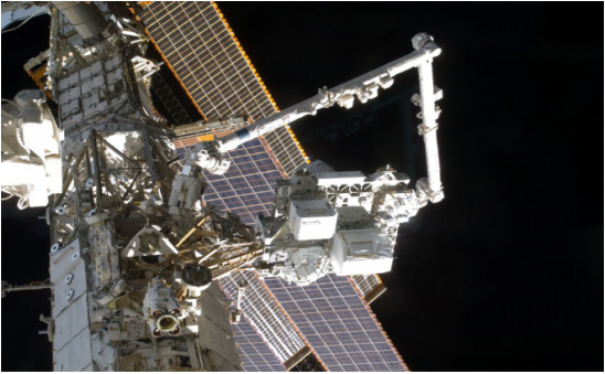
Canadarm2 mated ELC2 to the PAS on the ISS S3 truss, controlled by space shuttle and station crews during space shuttle mission STS-129.
