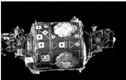
ISS Node 1, "Unity" module, and two pressurized mating adapters (PMAs) during space shuttle mission STS-88/ISS-2A
