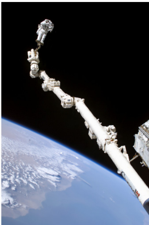
STS-114/ISS-LF1 mission specialist Stephen K. Robinson, anchored to a foot restraint on Canadarm2, participates in an EVA.
